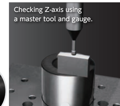
Calibration for touch probe using a master gauge.
