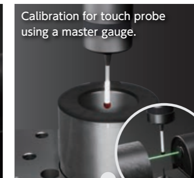
Checking Z-axis using a master tool and gauge.
